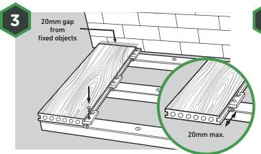
To secure the first board, use one Universal Clip and screw on every joist. Take a screw, place in the hole located in the Universal Clip and screw into the wooden joist. **Do not tighten at this stage.** Make sure the boards do not overhang the joist at the edge by **more than 20mm** and a **20mm expansion gap** should be left between the wall or other fixed objects surrounding the deck.
